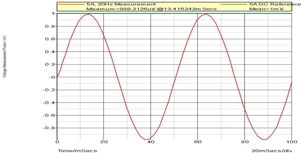
The legend indicates the mean value of the DC test signal and the peak value of the AC signal. The errors, about 0.1% are not discernable.
